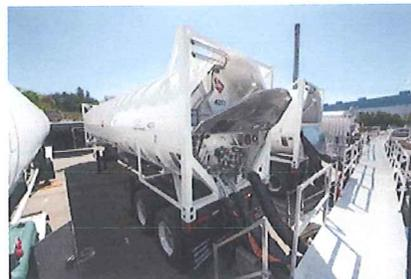
Tanker trailers filled with liquefied natural gas feed the Madison Paper Industries mill last fall. LNG is replacing 8 million gallons of oil a year at the mill, and saving the company millions of dollars. [click image to enlarge](#)
