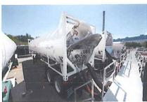
Tanker trailers filled with liquefied natural gas feed the Madison Paper Industries mill last fall. LNG is replacing 8 million gallons of oil a year at the mill, and saving the company millions of dollars.
