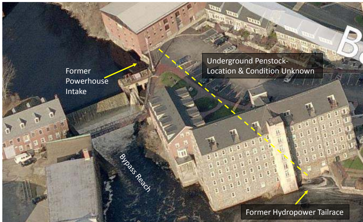
Figure 19: Aerial view of Macallen Dam's former hydroelectric works.
